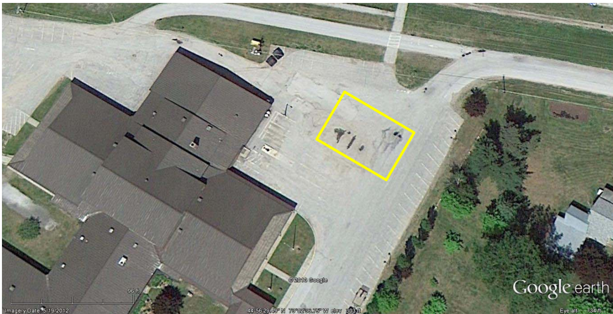
Figure 8. Low area in parking lot (shown in yellow) could be converted to stormwater treatment practice.
